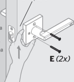
If the lever base will not sit flush on the door, use a flathead screwdriver to remove the alignment guide.
