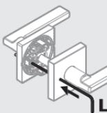
To unlock, insert the wrench and press with force.
