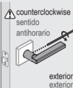
**B** Push up on lever base while tightening screws to keep latch horizontal and centered.
