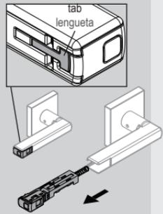
**B** Install (1) AAA battery provided. Instale (1) pila AAA incluida.
