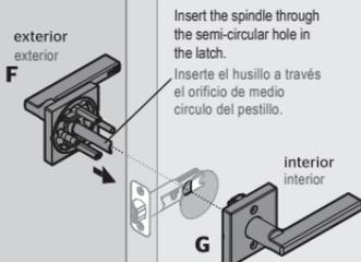
Insert the spindle through the semi-circular hole in the latch.
