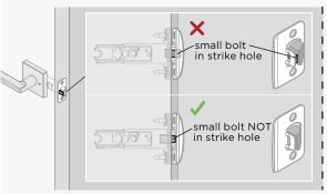
If latch is loose in the strike, adjust the strike tab so it grips the latch bolt better when the door is closed.
