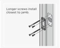
Note: The longer screws, 3" (76 mm) must be used to maintain highest security.
