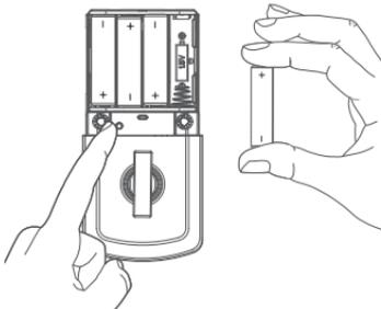
2. While still holding the Programming Button, insert the batteries.
