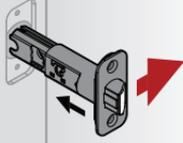
Install the bottom latch so that the slant of bolt faces in direction that door closes.
