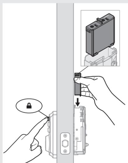
**C** The latch will retract and extend to learn the orientation of the door.
