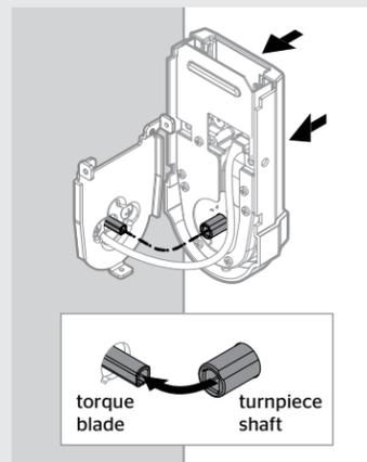
**G** Secure interior assembly with supplied screws.
