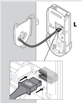
**E** Lay cable flat against the interior housing.
