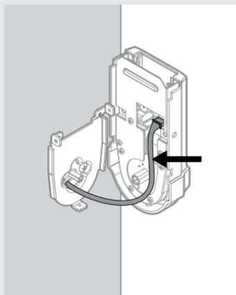
**F** Push turnpiece shaft onto torque blade.
