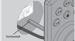
**F** Push the torque blade through the center hole in the mounting plate and send the cable through the bottom hole.
