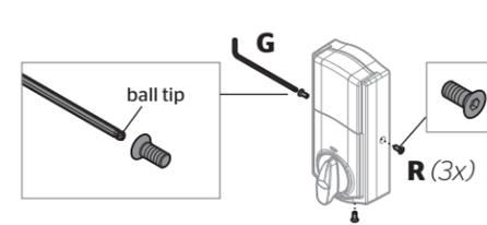
Keep "G" in a safe place, as you will need it to access the back panel for additional programming.
