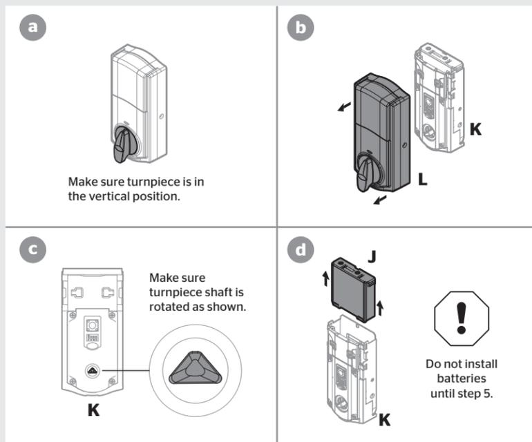
**B** Install interior assembly onto mounting plate.
