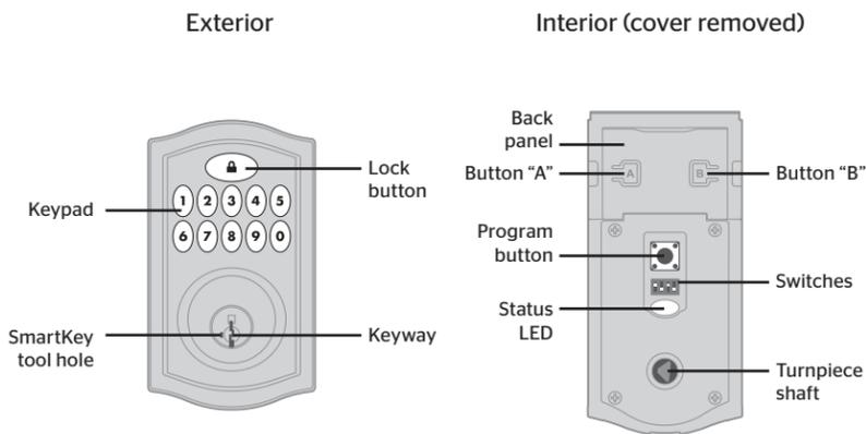
Note: When the cover is removed, the turnpiece shaft can be used to manually lock and unlock the door.
