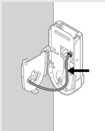
**F** Push turnpiece shaft onto torque blade.
