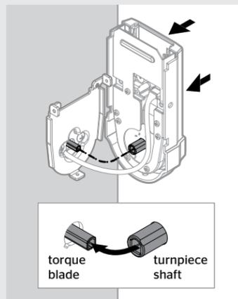
**G** Secure interior assembly with supplied screws.
