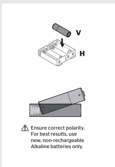
**B** Make sure the door is open, and insert the battery pack.
