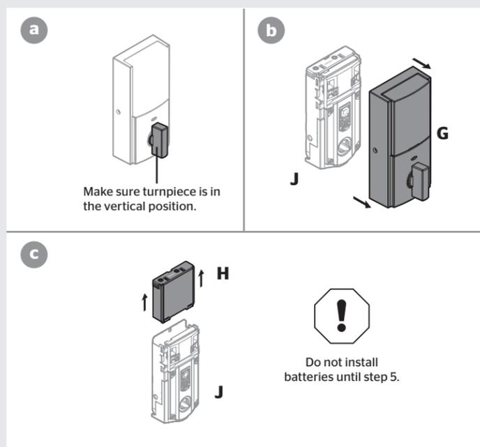
**B** Install interior assembly onto mounting plate.
