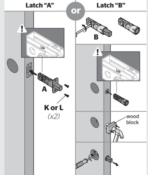
**C** Is the D-shaped hole centered in the door hole?
