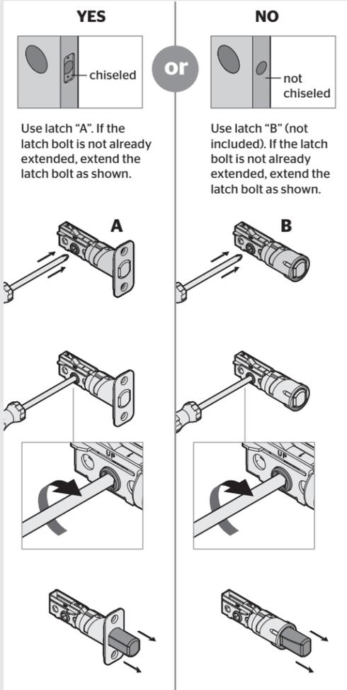
**B** Hold the latch in front of the door hole, with the latch face flush against the door edge.
