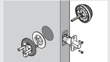
**C** Measure to confirm that the hole in the door is either 2-1/8" (54 mm) or 1-1/2" (38 mm).
