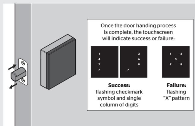
**D** If the touchscreen indicates a failure make sure that the cables are connected, the batteries are installed correctly, and attempt this procedure again.
