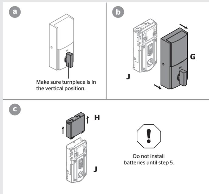
**B** Install interior assembly onto mounting plate.
