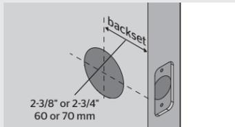
**E** Measure to confirm that the hole in the door edge is 1" (25 mm).
