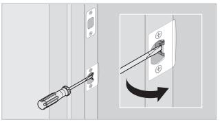
The lower latch and lower strike (for your knob or lever) are misaligned, putting too much load on the deadbolt latch.
