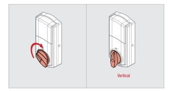
If the interior assembly is installed on the door, and the turnpiece cannot rotate to a vertical position, perform the door handing process. See the Installation and User Guide for more details.
