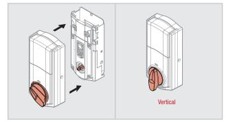
If it cannot rotate to the vertical position, use force to rotate the turnpiece clockwise until it clicks. The turnpiece should now be able to rotate to the vertical position.
