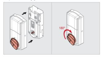
Align the turnpiece with the torque blade and reinstall the interior assembly on the door.
