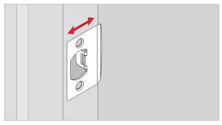
The hole in the door frame for the latch bolt is not drilled deep enough.
