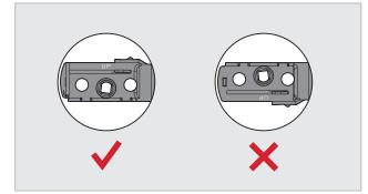
Reinstall the latch, making sure the word "UP" faces upward.
