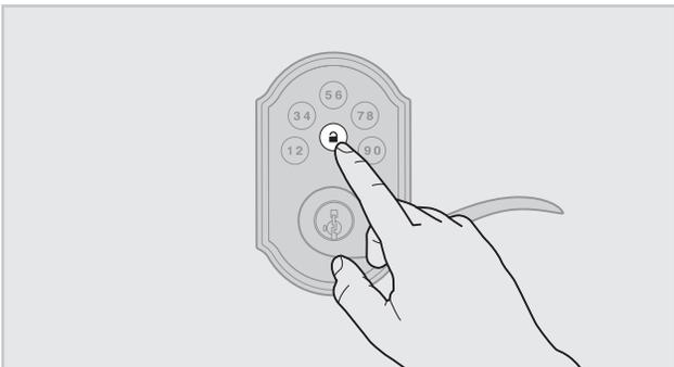
4. Press the Program button the number of times that corresponds to the user code position being programmed.
